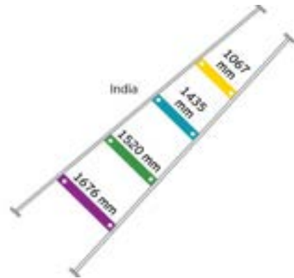
Figure 2-1: Gauges of Indian Rail
